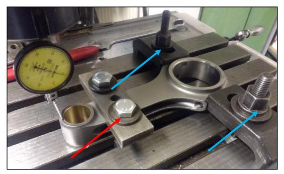
It's very important to check the parallelism of the small and big end of the rod. Don't tight the screw (red or blue arrow) too much, it'll bend or tipping the rod surfaces! Check it by a dial gauge! . I had a difference of 0,01mm between all rod surfaces, that's okay.
