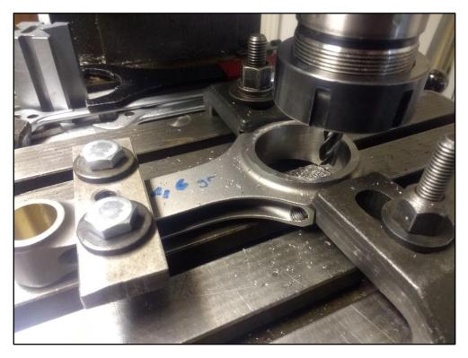
You need to turn the connecting rod on the milling maschine after removing 0,8mm. So the width will be 25,4mm.
