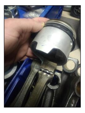
The only way to remove the old press fit piston pin ist to mill it down. Otherwise you will destroy the piston or the piston pin surfaces in the piston.
