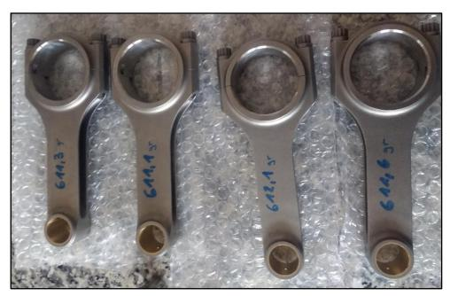
For milling the rods from 27,00mm to 25,40mm you need to mill 0,8mm from every side:
