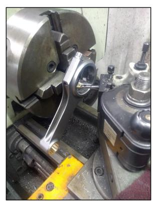
The last step is to turn a phase 1mm x 45°, because the original one doesn't exist anymore after milling. The phase is important to reduce friction between the rod and crankshaft.
